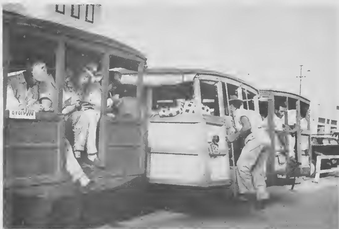
THESE TRUCKS are practically Lago land- marks. Each one can carry up to 35 men; they are simply truck bodies with seats and a roof built on the beds. They are practically indis- pensable to hundreds of employees who rely on them for transportation. E TRUCKNAN aki practicamente ta marcanan di Lago. Cada un por hiba 35 homber; nan ta simple curpa di truck cu un cashi y un dak built on the beds. Nan ta casi indispensable pa cien- tos di empleadonan cu ta depende ariba nan pa transportacion.
